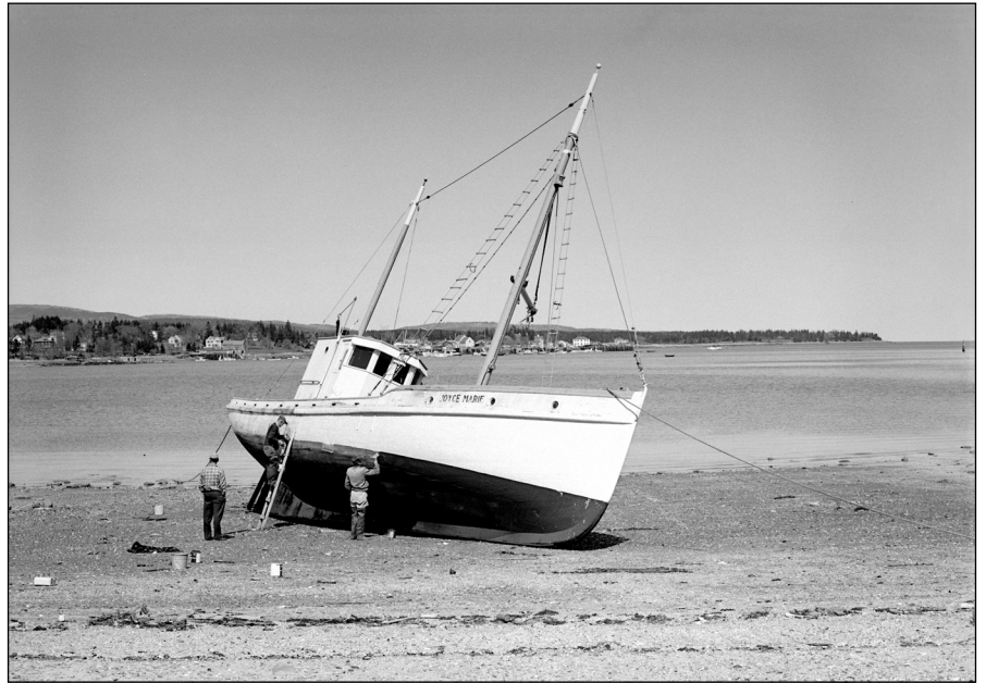
Sardine Carrier "Joyce Marie" Beached for Bottom Painting at Southwest Harbor - May 20, 1948 Photograph by W.H. Ballard Number 7873 - The Southwest Harbor Public Library Collection of Photographs
